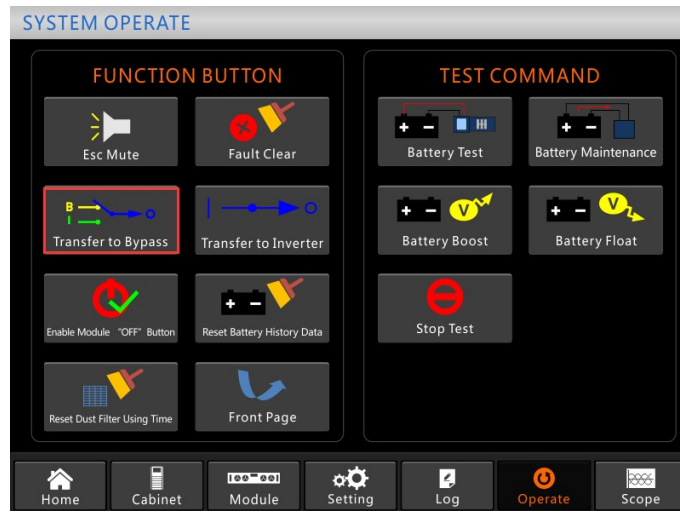
The operation interface for transferring to bypass
