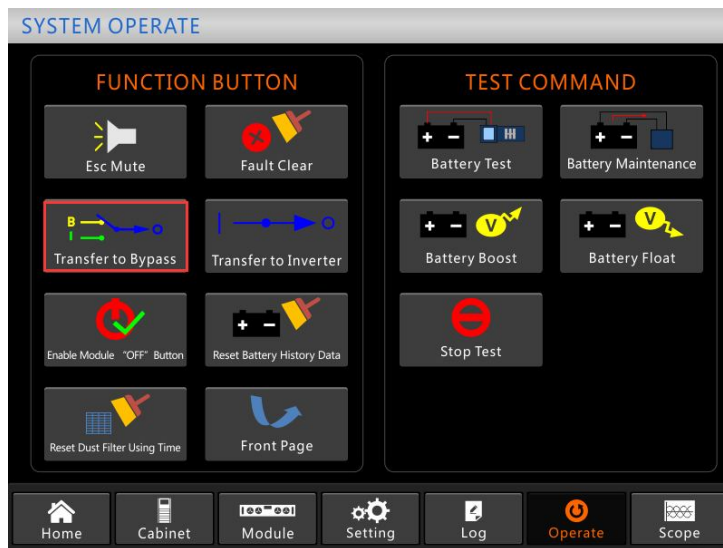
The operation interface for transferring to bypass
