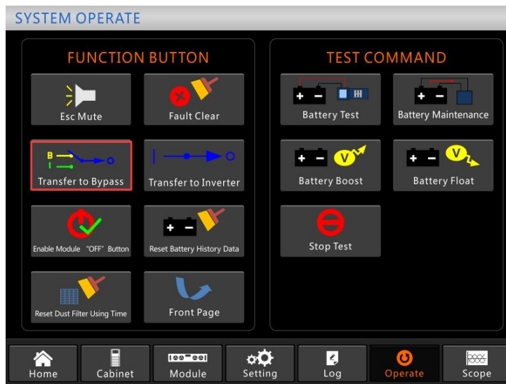
The operation interface for transferring to bypass
