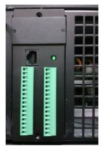
**Step 4**: Use RJ45 cable to connect UPS and equipment to implement remote monitoring and control.
