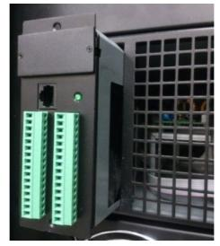
**Step 3**: The cover of extra communication card should attach close to STS module. Secure the extra communication card to the STS module chassis with 2 screws.
