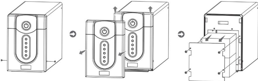
1. Ensure the UPS is turned off and disconnected from the main power.
