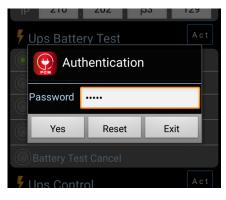
Authentication is required and only pops up after you connected to the UPS and try to do **Battery Test**, **UPS Control** or **UPSMON PRO Control**.
