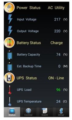
Status panel displays the status of the connected UPS, including the Power status, the Battery Status and UPS Status.
